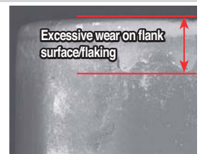
Existing grade (K15)
