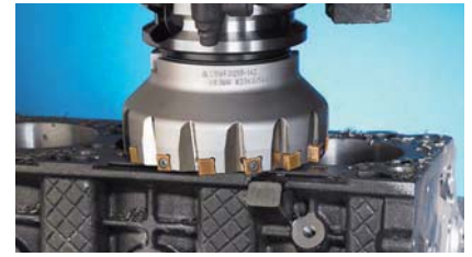
Roughing for cast iron
