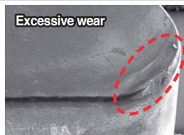
Existing grade (K10)
